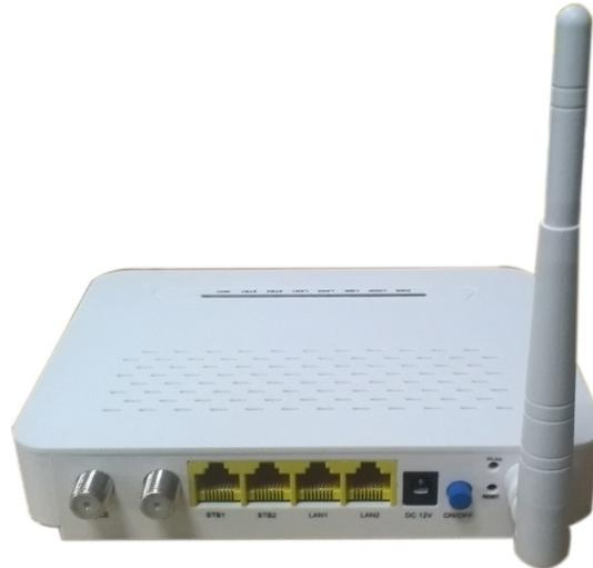
HV5204WL is the EOC slave based on HomePlug AV solution for Ethernet access over coax.
